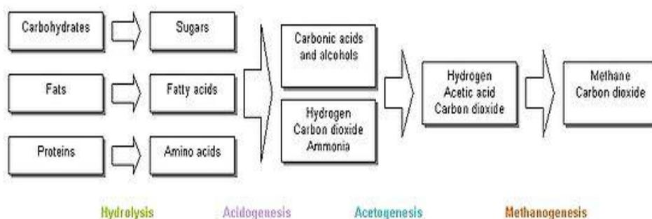
The raw biogas produced is dried and hydrogen sulphide and other trace substances removed and after cleaning, the biogas is upgraded to biomethane or combusted in a combined heat and power (CHP) plant to generate electricity and heat simultaneously. The digested sludge is dewatered and the water reintroduce into the treatment plant while the remaining undigested matter used for organic fertilizer. <sup>(4)</sup>
